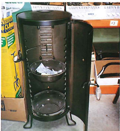
The vertical drum smoker with adjustable rack. The main disadvantage with this smoker is the full door will let all the smoke out when turning the grain or adding fuel. The cost is approximately $100.
